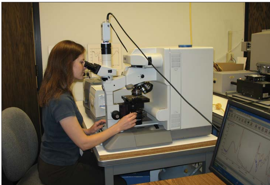
Winterthur associate scientist Catherine Matsen performing an infrared spectroscopy (FTIR) analysis of an eighteenth-century painted dower chest sample.
